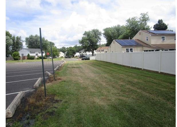
A rain garden can be installed adjacent to the parking lot to capture, treat, and infiltrate runoff from the parking lot. Two more rain gardens can be installed at the front of the building to collect water from downspouts. A preliminary soil assessment suggests that more soil testing would be required before determining the soil's suitability for green infrastructure.
