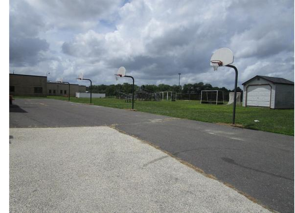
The basketball courts to the north of the building can be converted to pervious pavement to capture and infiltrate stormwater runoff from the surrounding paved areas. A rain garden can be installed in the turfgrass area on the west side of the building to capture, treat, and infiltrate stormwater runoff from the roof. A preliminary soil assessment suggests that more soil testing would be required before determining the soil's suitability for green infrastructure.
